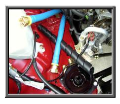
5) Attach the center hose from the filter unit to the tapered adapter fitting in the center hole on the base unit. Thread sealant is <u>not</u> needed here, as this is a compression type fitting. Tighten securely (7/8" open-end wrench). NOTE: refer to chart on page 5 labeled "Torque Specifications for Aluminum Fittings" for proper tightening instructions.
