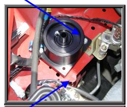
4) Next, you are going to drill the 2<sup>nd</sup> mounting hole (in the tab that sticks out toward the engine). Position your base unit as shown, and using it as a template, center-punch where you will drill the mounting hole in the tab (you can feel the hole that is already there from underneath the tab). Note: on '99 & 2000 cars this hole is already there – lucky you, no drilling required!
