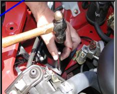
5) Drill ¼" hole through. Insert 2<sup>nd</sup> M6 x 30mm bolt with washer, add 2<sup>nd</sup> rubber isolator mount (thick rubber washer) between base unit and body, and secure with Nyloc<sup>®</sup> nut and flat washer at bottom. *TIP: Hold a moistened (with water) paper towel or cloth under the tab when drilling the hole – this will catch the drill bit chips.*
